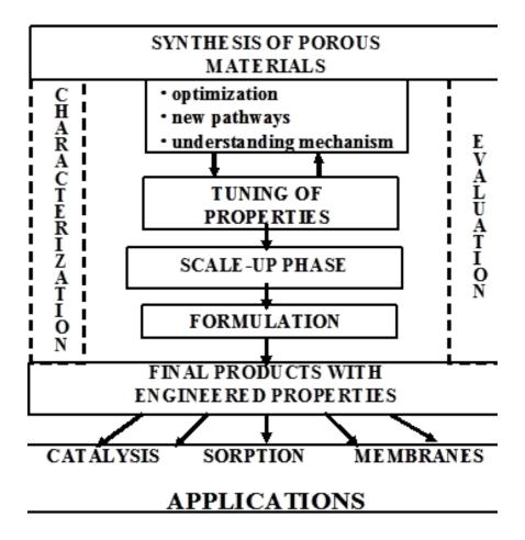
Materials with very narrow pores in the nano-scale range, i.e. from ca. 0.1 to 100 nm, are commonly referred to as **nanoporous materials.** Note that the lower end of this range, viz. from ca. 0.1 to 1 nm, coincides with the dimensions of the vast majority of molecules. The similarity of molecular dimensions and pore widths forms the basis for some unique and most striking applications of nanoporous materials in modern separation processes and heterogeneous catalysis.
